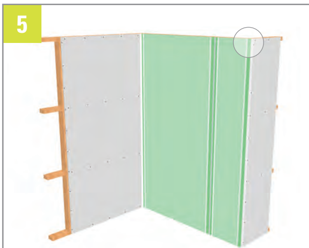
Install external corner jointer
