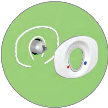
Peel back protective film from front face of EnduraPanel, to 25mm beyond the outer edge of the shower mixer's installed perimeter.
