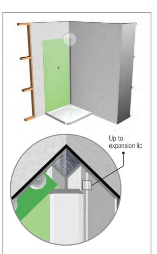
Peel back protective film from front face of EnduraPanel, 25mm from the edge to be inserted into internal corner jointer.
