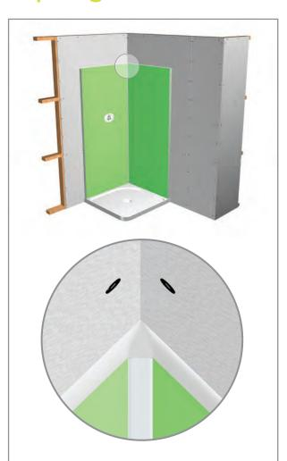
In line with BRANZ recommendation, we suggest that silicon be applied to the top of EnduraPanel. This is to prevent any moisture penetrating down behind the lining. Special attention should be paid to the top of the internal corner jointer and anti-fracture membrane areas. See illustration, above.
