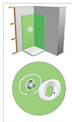
Peel back protective film from front face of EnduraPanel, to 25mm beyond the outer edge of the shower mixer's installed perimeter.
